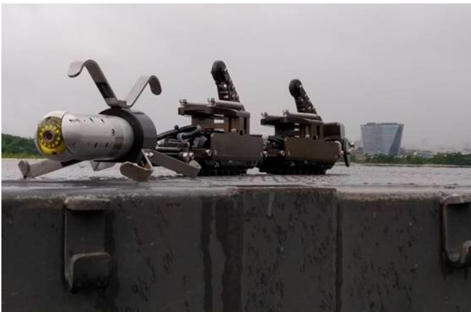
Figure2: VT-1100, medium class crawler, designed for RVI and NDT in small diameter pipes.
