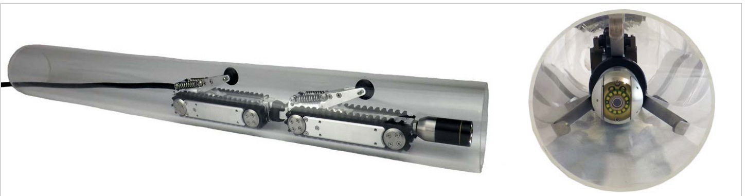
Figure 3: Designed to enter an opening as small as 51 mm (2in) up to 305mm (12in).
