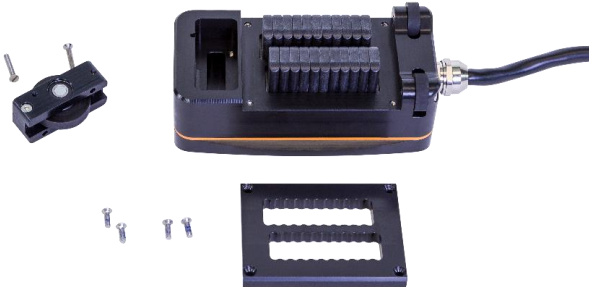
Figure 28. The encoder and the removable frame can be dismantled to clean the probe. Supporting wheels can also be removed if necessary
