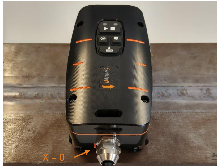
Figure 7. Scan position x=0 aligned with the marker line on the probe side
