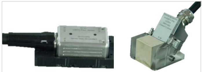
Figure 3: DLA probe (2 x 64-element) designed for pitch-catch inspections & linear array (64-element) with curved active elements provides a small focal beam (~1mm) along both the active and passive planes.
