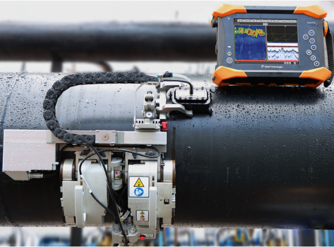
Figure 1: PAUT corrosion mapping with Navic scanner and Mantis.
