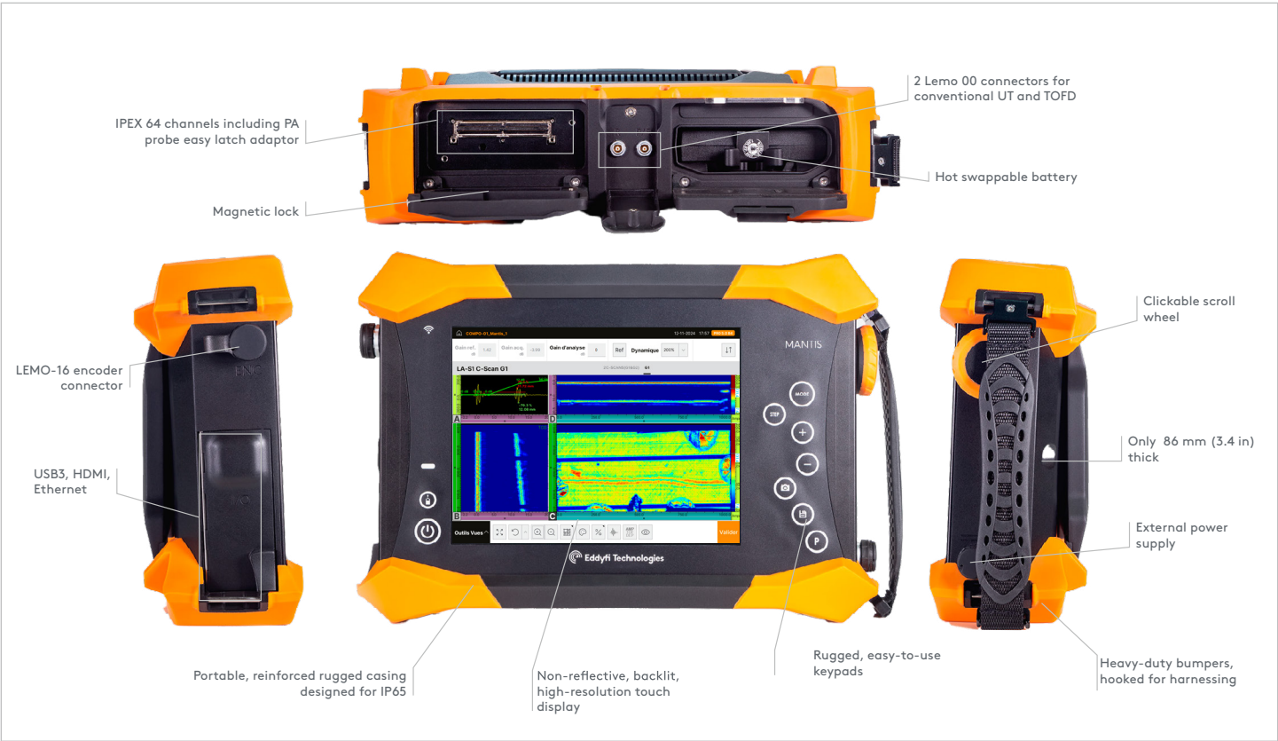
Figure 4: Annotated breakdown of Mantis showing its key features.
