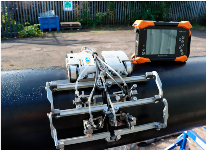
Figure 6: Navic scanner with Mantis for pipe inspection.
