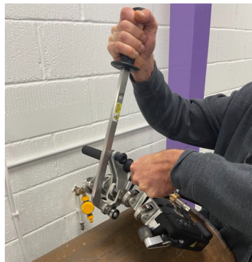
Figure 23: Pipescan HD Deployment 03
