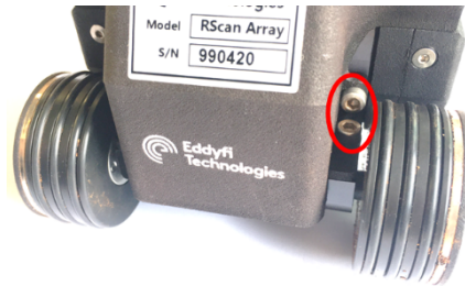
Figure 12: Front handle front bolt location
