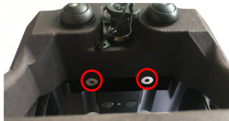
Figure 13: Front handle rear bolt location
