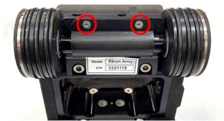
Figure 11: Front handle dust cover screw location
