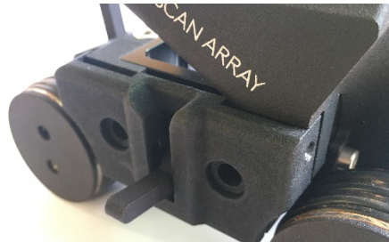
Figure 20: Prising off the right side cover
