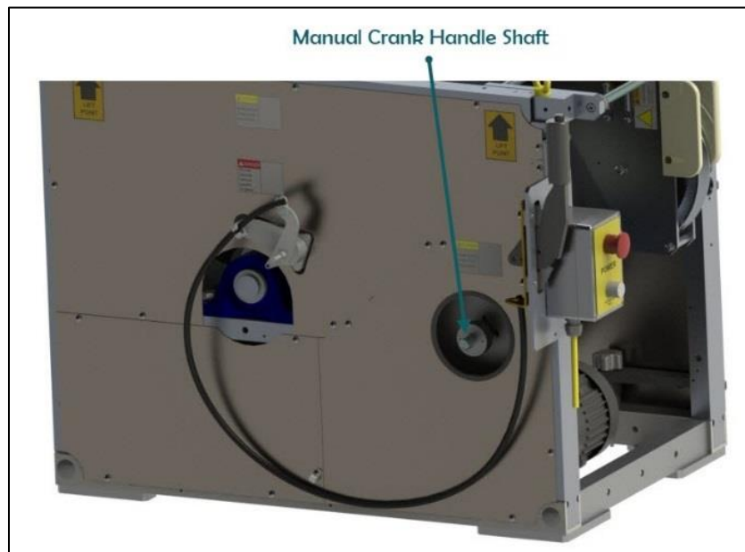
FIGURE 14: MANUAL CRANKING SHAFT POSITION
