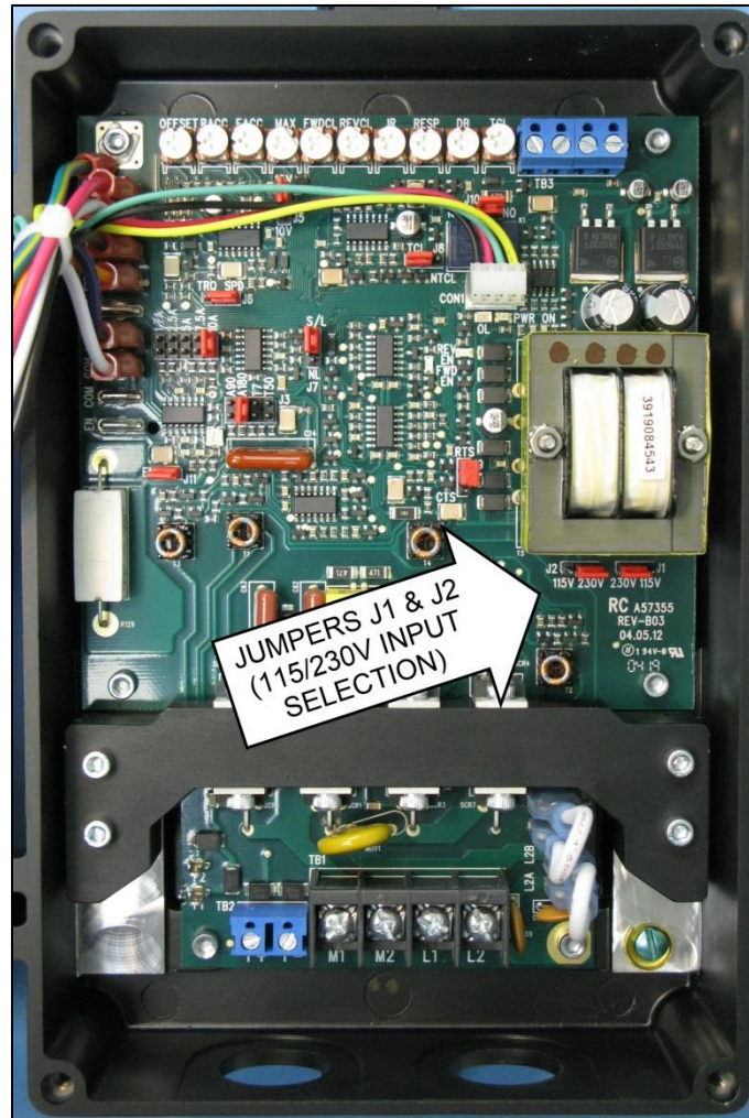
FIGURE 5: LINE VOLTAGE SELECTION, JUMPERS J1 AND J2
