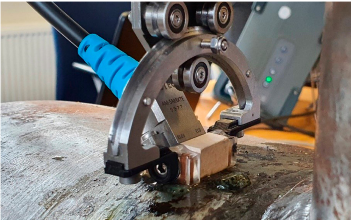
Figure 4: PAUT probe 2D Matrix Array mounted in nozzle scanner
