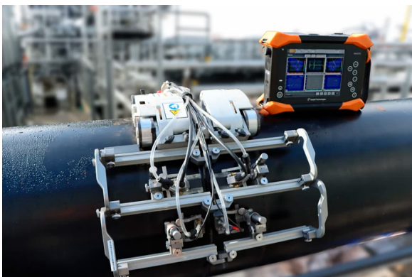
Figure 1: Weld inspection of pipework utilizing Nav2 and Mantis.
