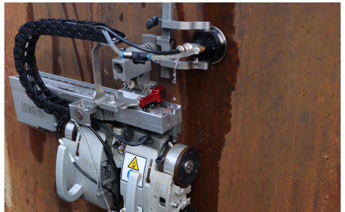
Figure 3: NAV2 conventional SCUT corrosion mapping configuration.
