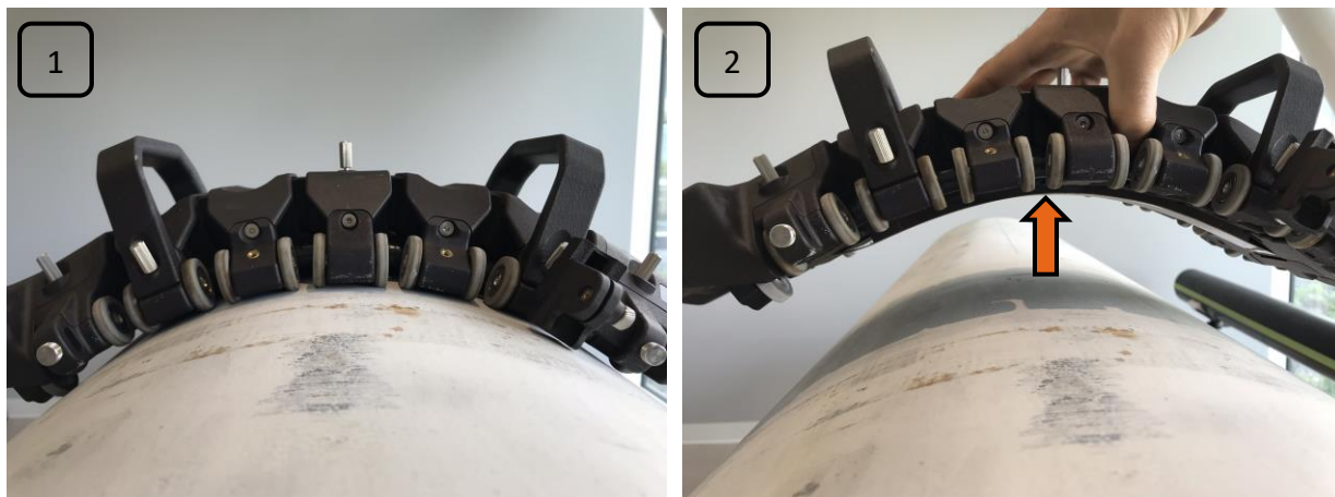
Figure 20. Spyne lift-off calibration: 1) Null the Spyne on a clean section of the inspected surface, with the whole length of the probe in good contact with the surface; 2) Start an acquisition and slowly lift the probe in the air.
