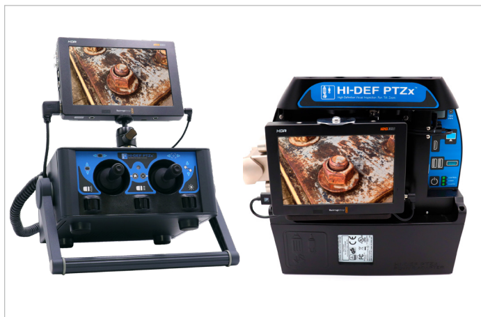
Figure 6: Modular (left) and integrated (right) camera control units.
