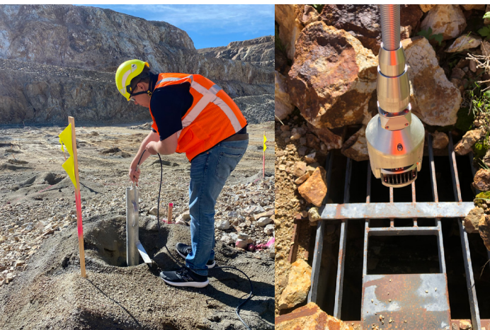
Figure 2: Hi-Def PTZx 3.0 in the surface mining industry. The camera is lowered down a drilled hole to an underground void (left), and a mine shaft with crib supports (right).
