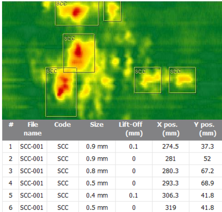
Figure 13. Summary table displayed on the first page of the report, containing information about all the defects that were reported in the current inspection. This is usually followed by individual screenshots and information of all the reported defects.
