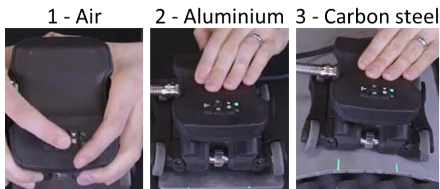
Figure 3. The three probe calibration steps
