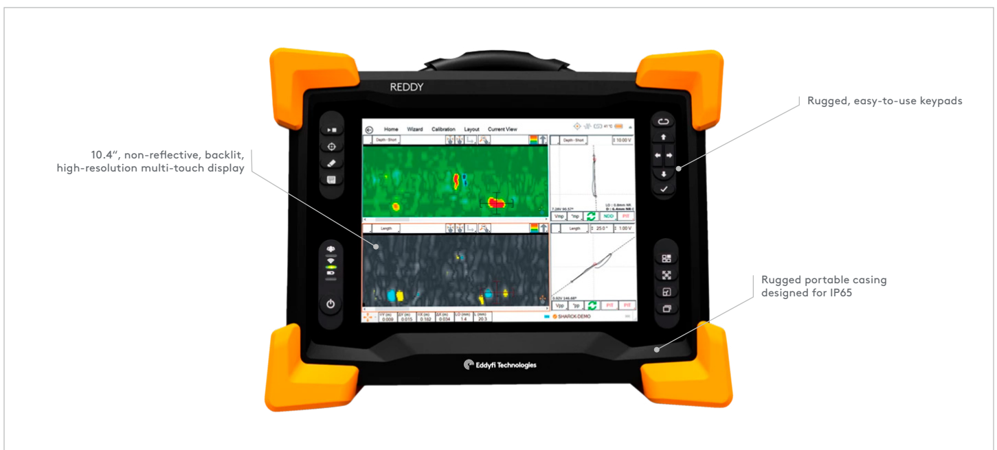
Figure 1: Annotated breakdown of Reddy showing its key features.
