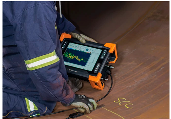
Figure 5: Detecting and assessing stress corrosion cracking in base metal using I-Flex™ paired with Reddy.
