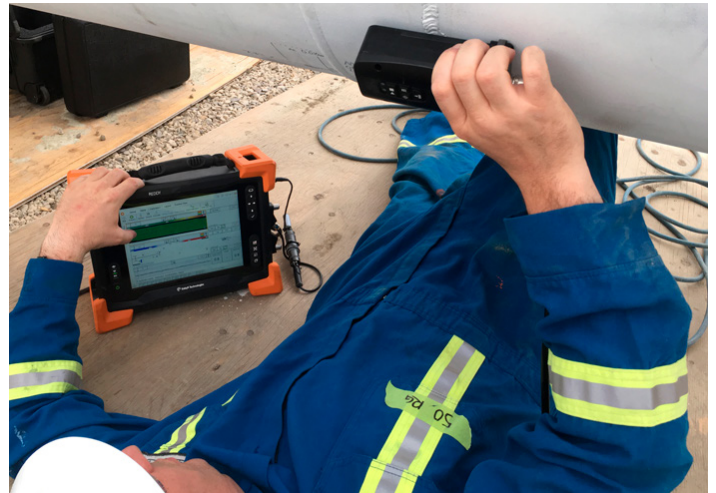
Figure 2: Detecting and sizing cracks in carbon steel welds using the Shark™ paired with Reddy.
