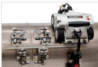
Figure 6 and Figure 7: Automated chain scanner for non-ferrous & ferrous pipe inspection.
