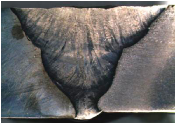
Figure 1: Anisotropic coarse-grain structure in austenitic materials
