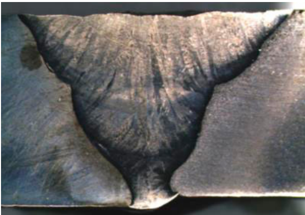
Figure 1: Anisotropic coarse-grain structure in austenitic materials
