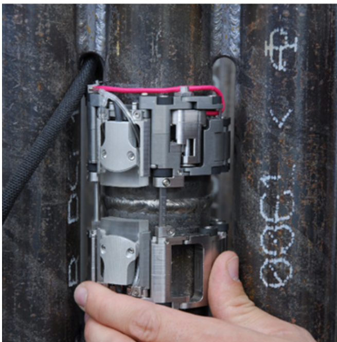
Figure 1: CIRC-IT examines the welds of small pipe diameters.
