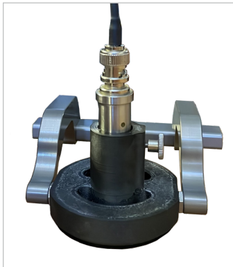
Figure 5: Single crystal probe with a local immersion water column.
