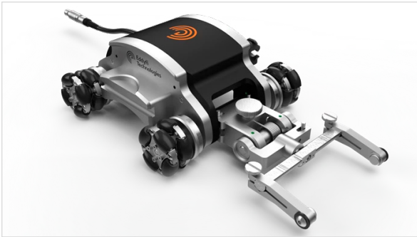
Figure 10: Semi-automated NDT Sweeper for corrosion and weld inspections.
