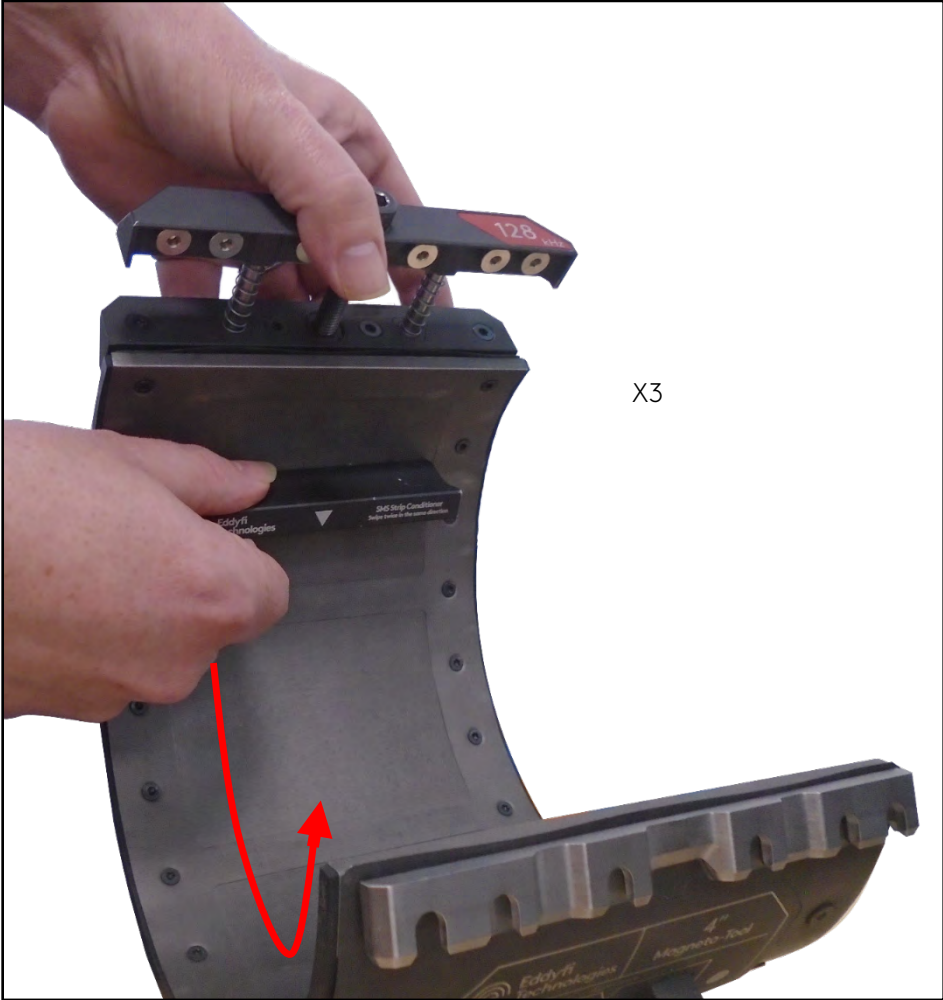
Position the collar at the selected test location, taking note of the forwards orientation of the collar.
