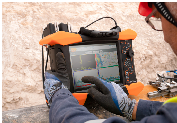
Figure 2: In-field inspection using Gekko.
