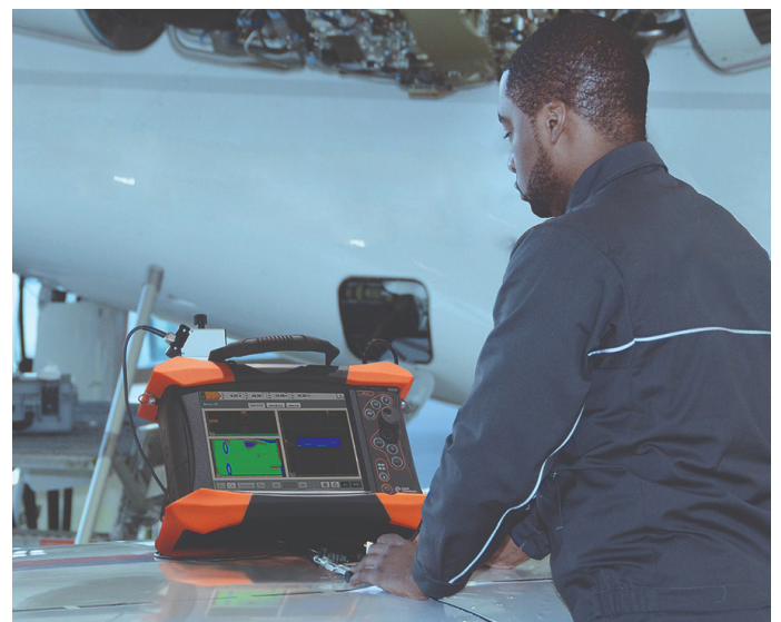
Figure 4: Gekko performs aerospace composite material inspection.
