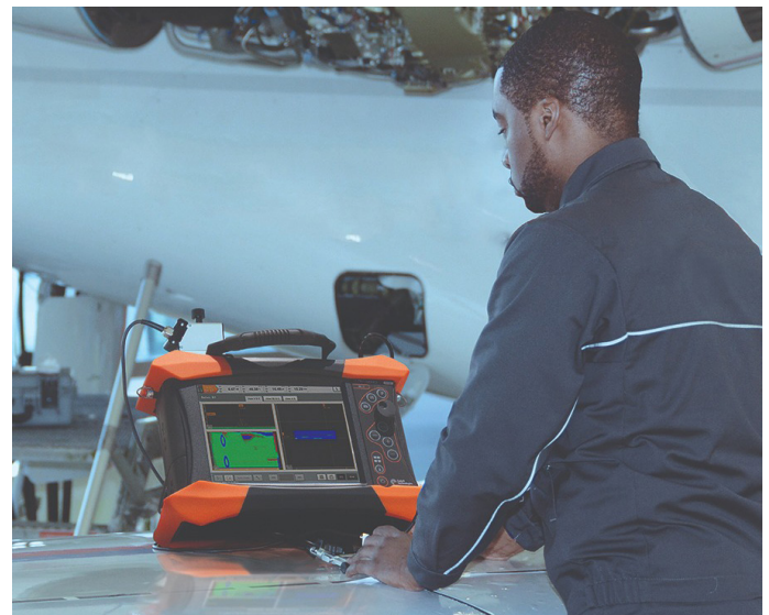
Figure 4: Gekko performs aerospace composite material inspection.
