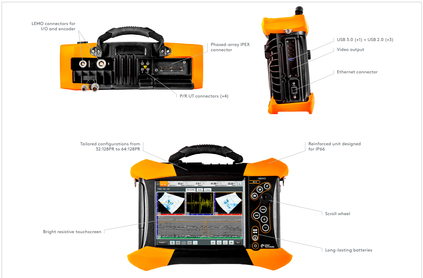
Figure 1: Annotated breakdown of Gekko showing its key features.
