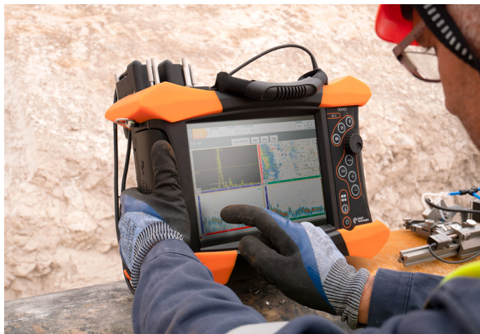
Figure 2: In-field inspection using Gekko.
