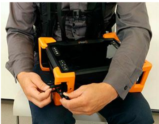
Figure 8-9 Securing anchor strap
