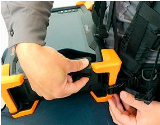
Figure 8-14 Closing battery compartment door.
