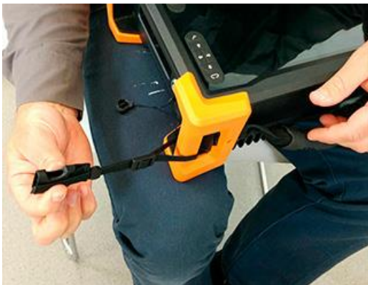
Figure 8-10 Alternative method of securing anchor strap to bumper
