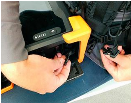
Figure 8-12 Slipping male buckle through bumper
