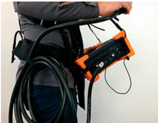
Figure 8-17 Belt-slinging probe cable
