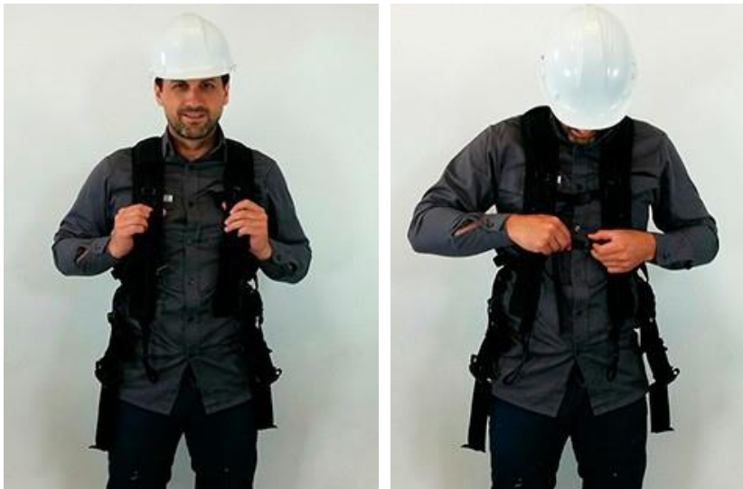
Figure 8-4 Securing the chest straps
