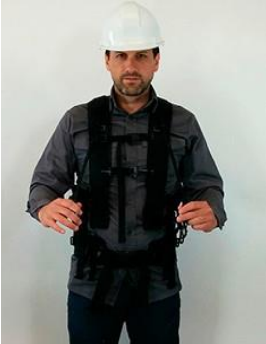
Figure 8-6 Shoulder anchor straps
