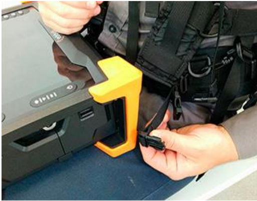
Figure 8-11 Anchor strap on harness belt
