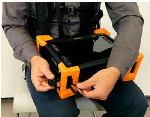
Figure 8-8 Sliding strap loop through bumper hook
