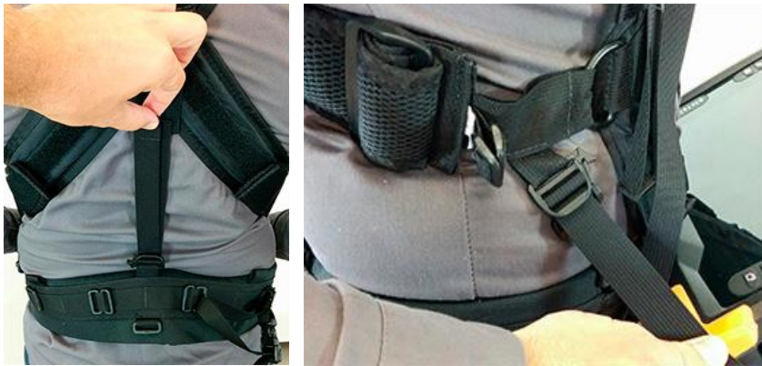
Figure 8-3 Adjusting the belt's height
