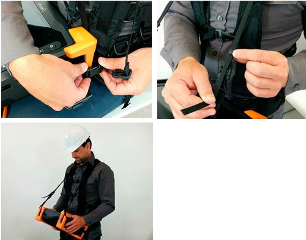
Figure 8-13 Mating battery compartment side anchor strap
