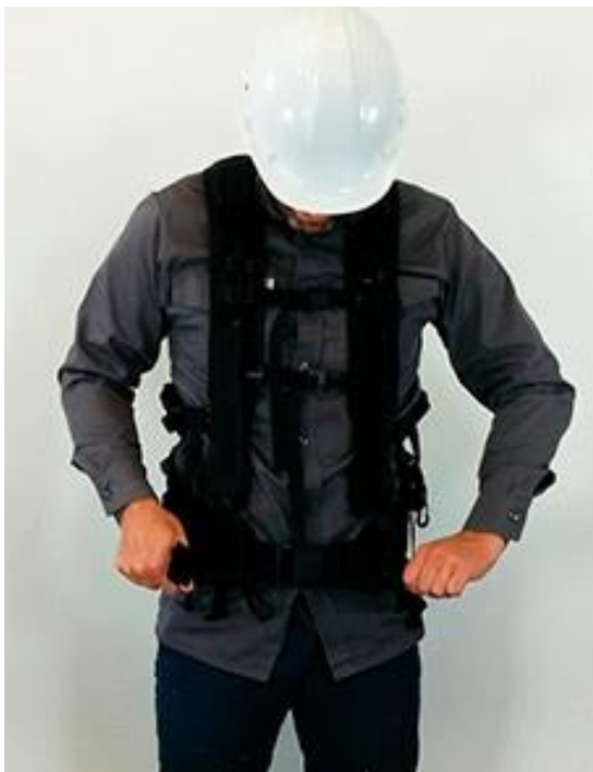
Figure 8-5 Securing the belt
