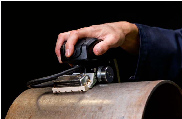
Figure 1: PaintBrush2 can inspect curved surfaces and pipes with a diameter as small as 100mm (4in).
