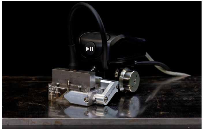
Figure 3: PaintBrush2 with NW1 probe for inspection of composites.
