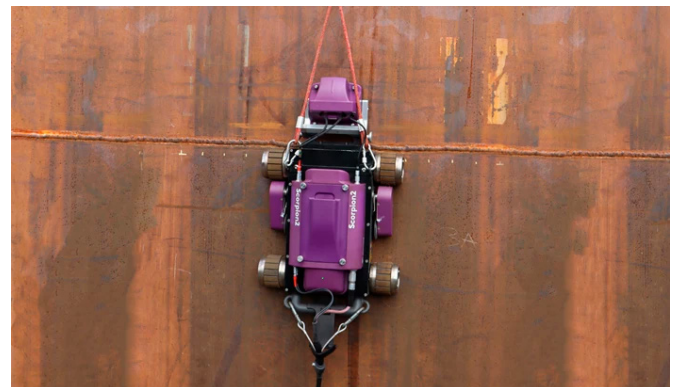
Figure 4: Tank inspection using Scorpion2.
