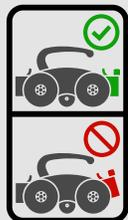
**WARNING!** **ONLY USE ACTUATED PROBE LIFTS WHEN SWIVEL MOUNT IS LOCKED IN THE HORIZONTAL POSITION.**
