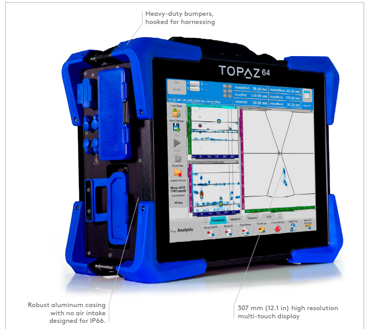
Figure 1: Annotated breakdown of TOPAZ64 showing its key features.
