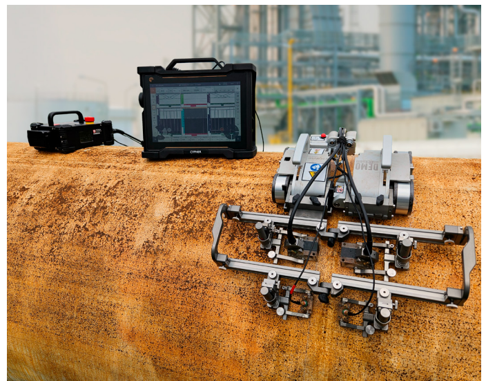
Figure 6: Automated solution featuring NAV2 scanner.
