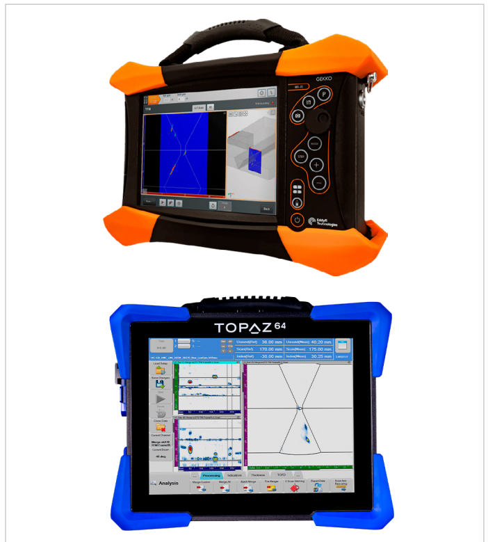
Figure 3: Powerful Instrumentation - Full inspection in one go with the multi-mode capability, TOPAZ64 can support two FMC acquisitions, up to 4 TFM per FMC, + PA + TOFD all at the same time.
