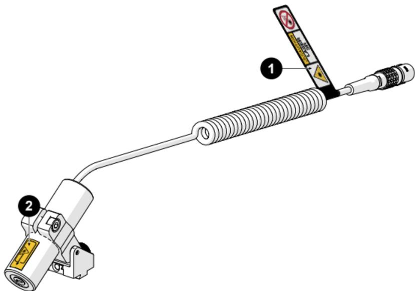
Fig. 1 - Optical guide safety label locations
