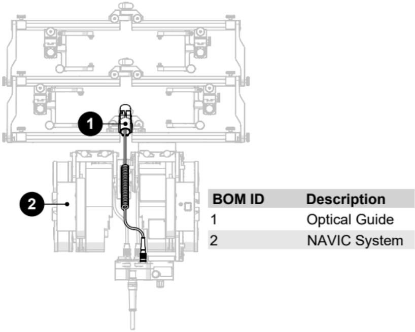
Fig. 12 - Optical Guide mounted to a pivoting probe holder frame
