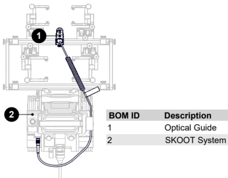
Fig. 14 - Optical Guide mounted to a low profile probe holder frame
