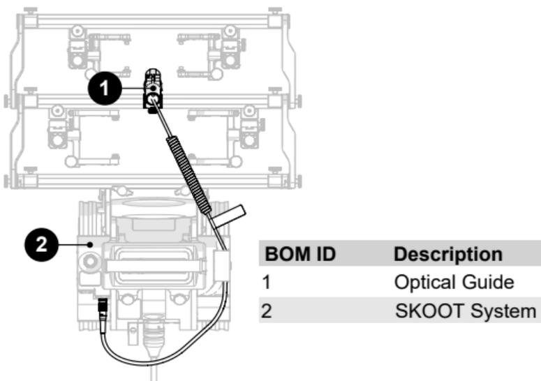
Fig. 13 - Optical Guide mounted to a vertical probe holder frame
