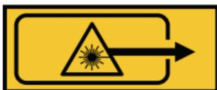
Fig. 2 - Laser aperture label
