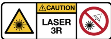
Fig. 3 - Laser radiation label
