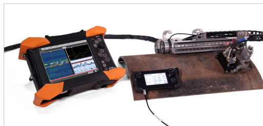
Figure 5 and 6: Automated crawler for corrosion and weld inspection. Handles removable.
