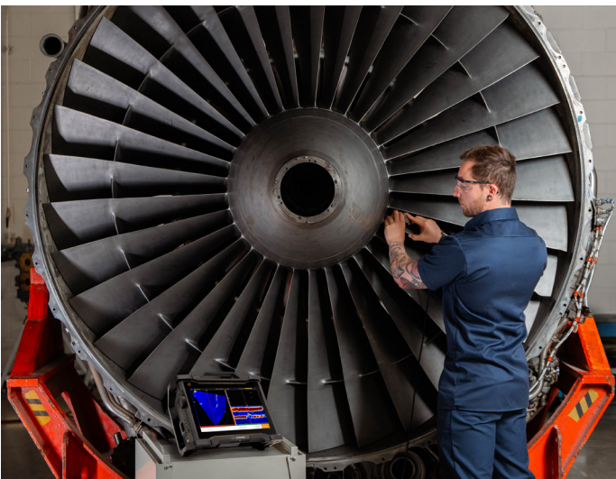
Figure 3: Turbine inspection using Cypher, PAUT probe and wedge configuration.
