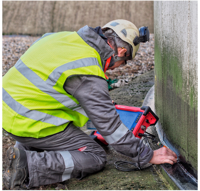
Figure 2: Amigo2 for ACFM weld inspection.
