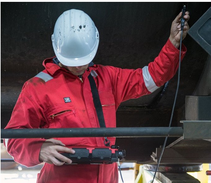
Figure 4: Sensu 2 ACFM probe with the Amigo 2 for rail tank car weld inspection.
