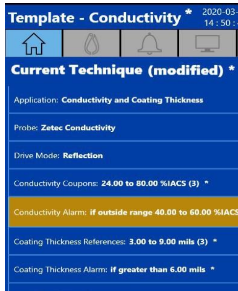
Figure 4-14 Conductivity and thickness alarm
