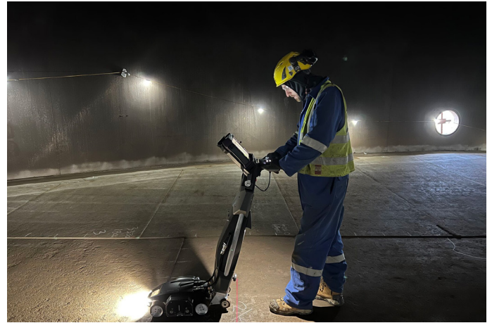
Figure 8: FloormapX MFL tank bottom inspection.
