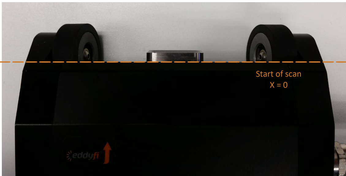
Figure 50. Scan position x=0 aligned with the front of the probe
