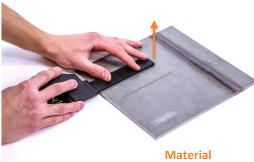
Performing a lift-off with the I-flex probe
