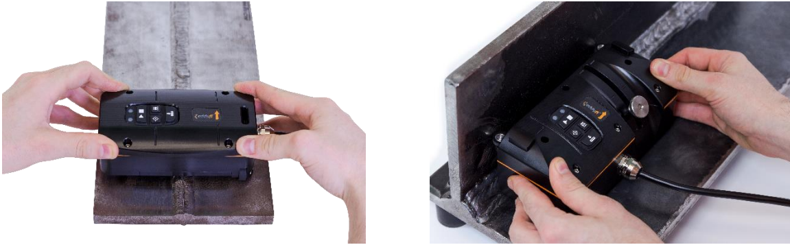
Figure 7. Sharck probes on carbon steel weld
