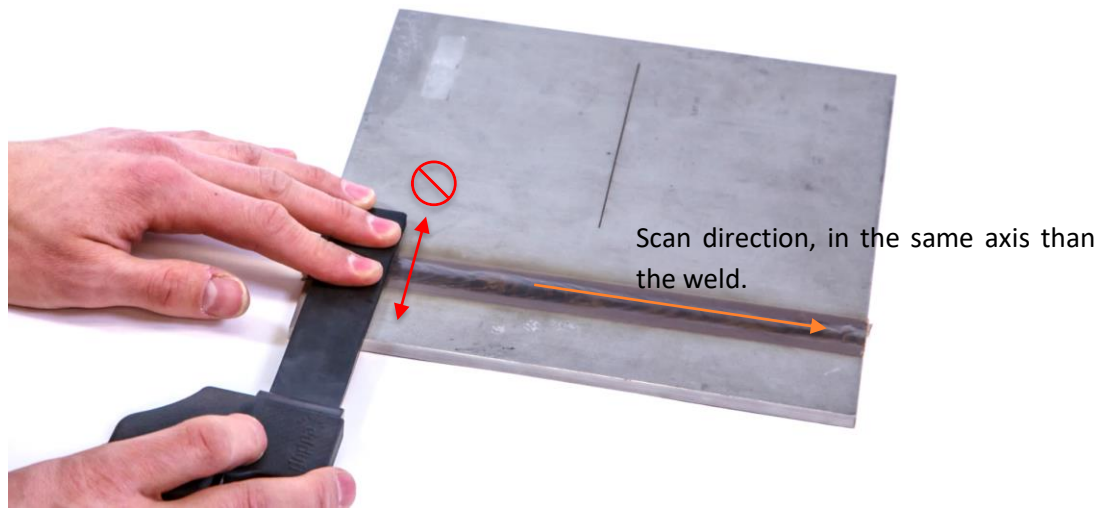
Scanning a weld with the I-Flex probe
