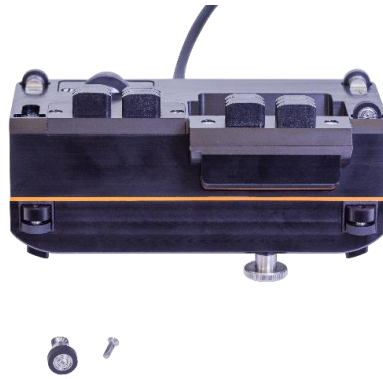
Figure 32. Guiding and supporting wheels can also be unscrewed if it is necessary to clean them
