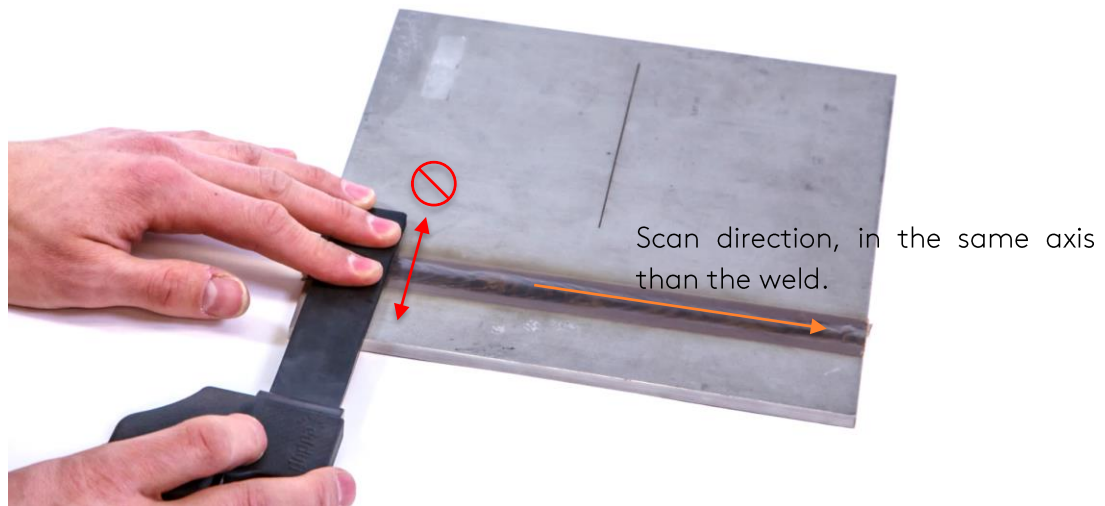
Scanning a weld with the I-Flex probe
