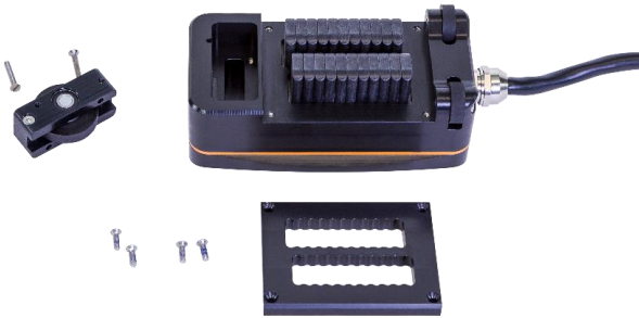
Figure 72. The encoder and the removable frame can be dismantled to clean the probe. Supporting wheels can also be removed if necessary
