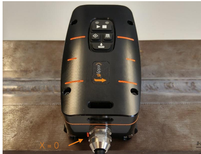
Figure 51. Scan position x=0 aligned with the marker line on the probe side
