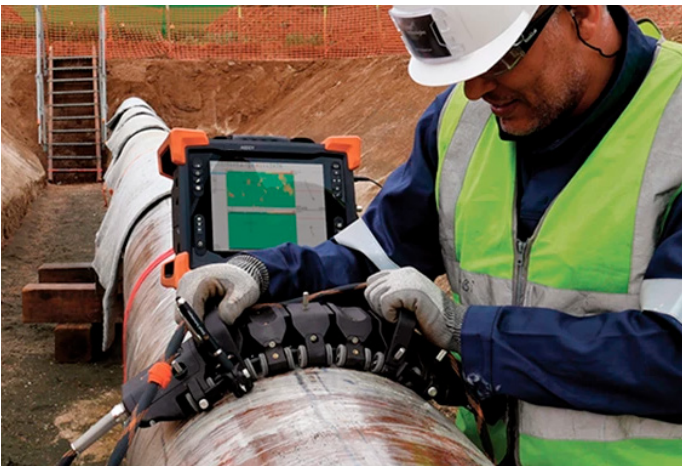
Figure 3: Operator performing in-field data analysis during a pipeline inspection using a Spyne™ ECA probe, Reddy® instrument, and Magnifi GO software.
