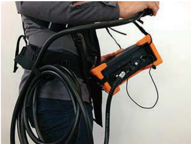
Figure B-17 Belt-slinging probe cable
