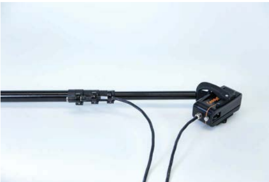
Figure C-5 Running PEC probe cable through pole hoops
