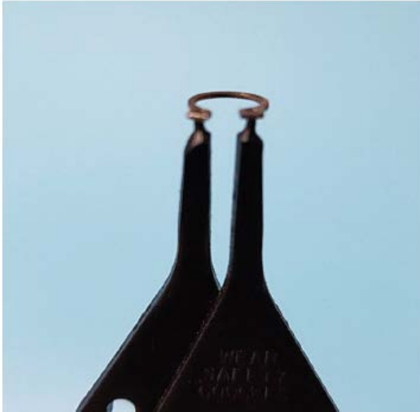
Figure 7-3 Clamp ring sitting on plier
