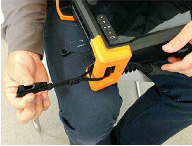
Figure A-10 Alternative method of securing anchor strap to bumper
