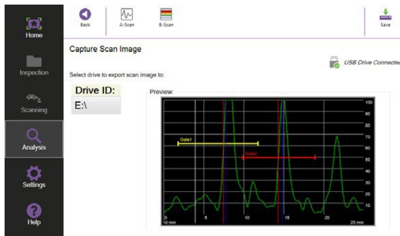
Figure 6–18 Capture A-Scan image
