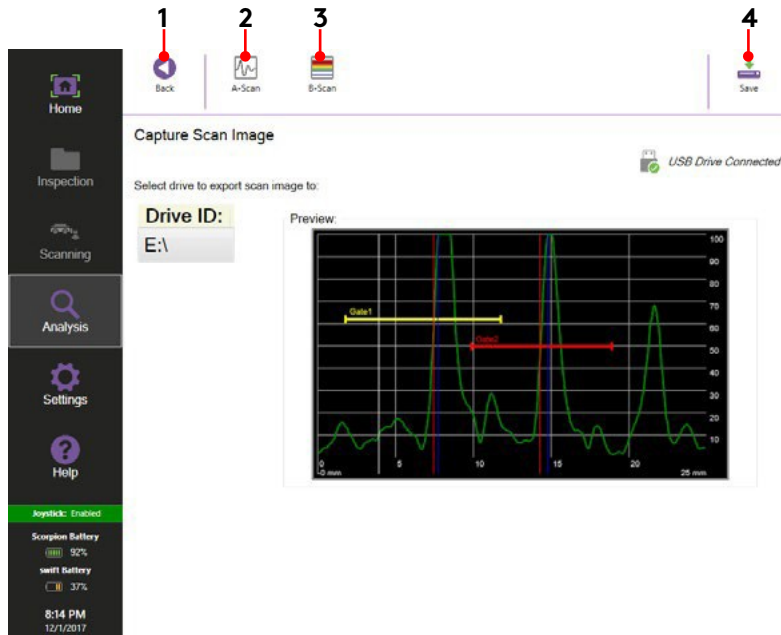
Figure 4–11 Capture scan window
