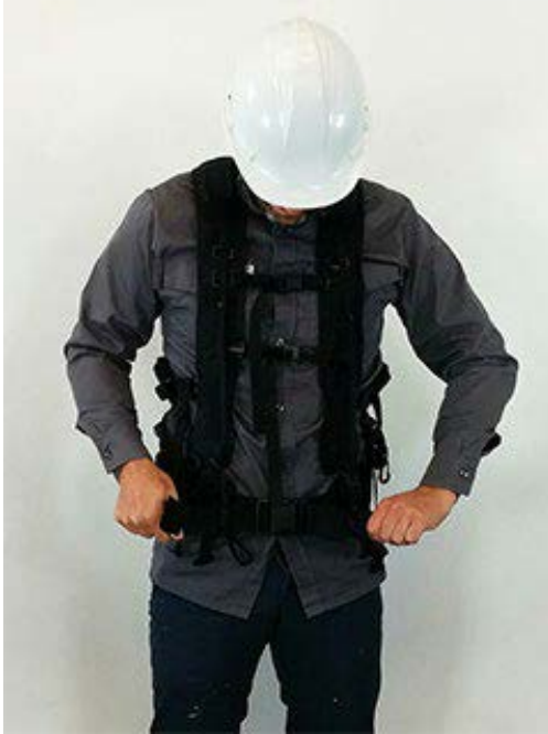
Figure A-5 Securing the belt
