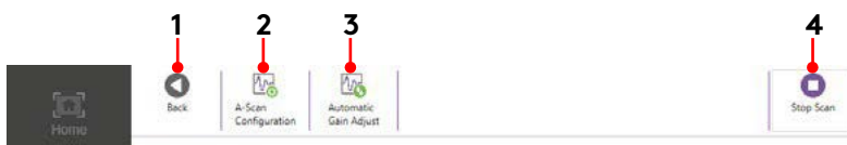
Figure 4–7 Manual scan toolbar
