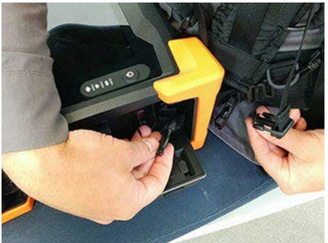
Figure A-12 Slipping male buckle through bumper
