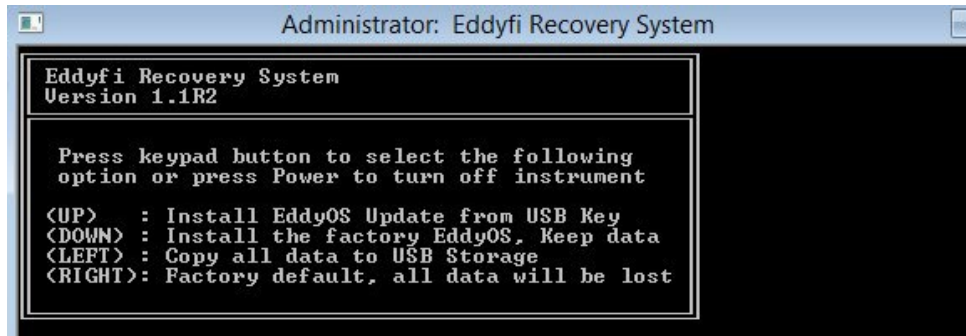
Figure 7-2 System recovery interface
