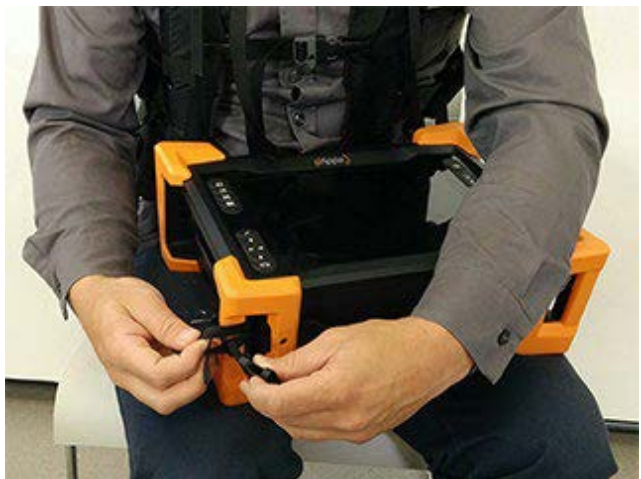
Figure A-9 Securing anchor strap
