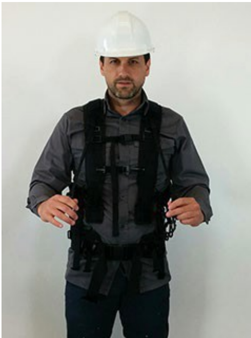
Figure A-6 Shoulder anchor straps
