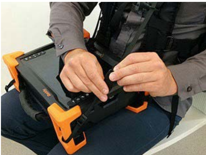
Figure A-15 Mating shoulder anchor strap
