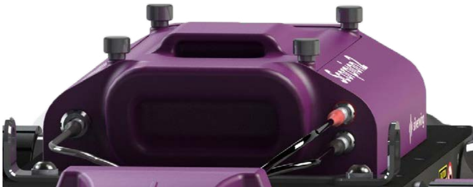
Figure 5-2 Scorpion2 front connectors
