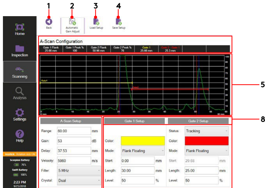
Figure 4–8 A-Scan configuration window
