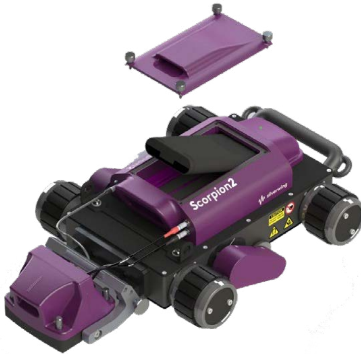
Figure 2-5 Scorpion2 inserting batteries
