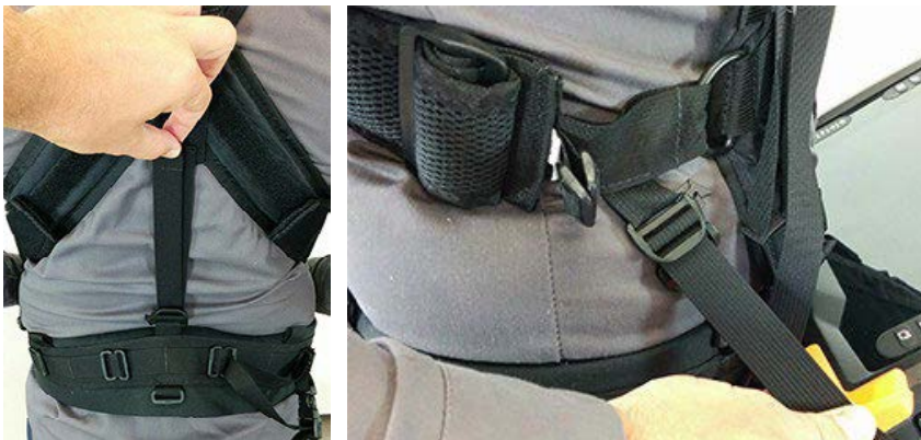
Figure A-3 Adjusting the belt's height
