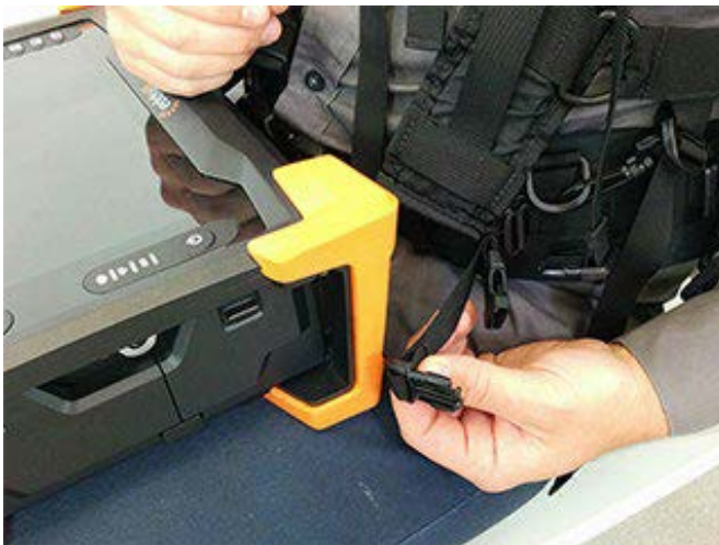
Figure A-11 Anchor strap on harness belt
