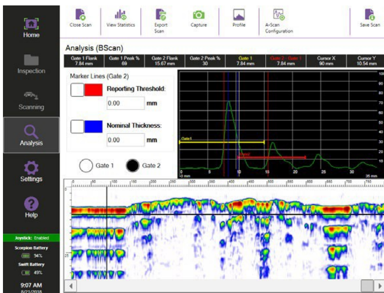
Figure 6–13 Analysis (B-Scan) window
