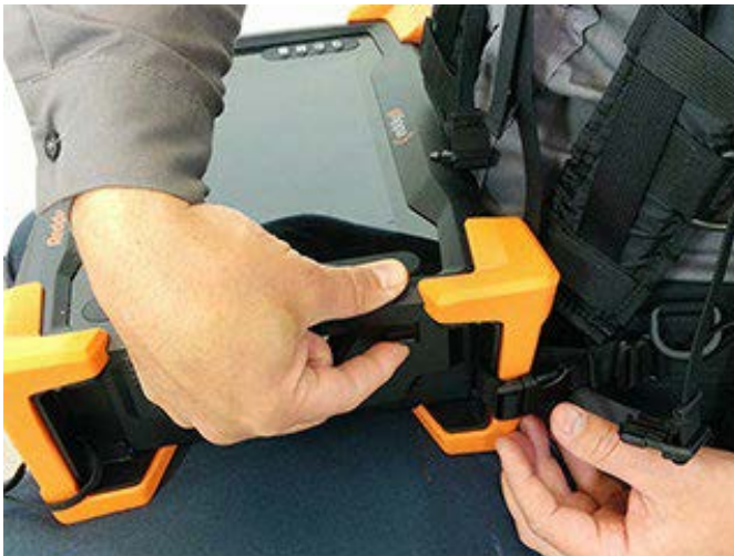
Figure A-14 Closing battery compartment door.
