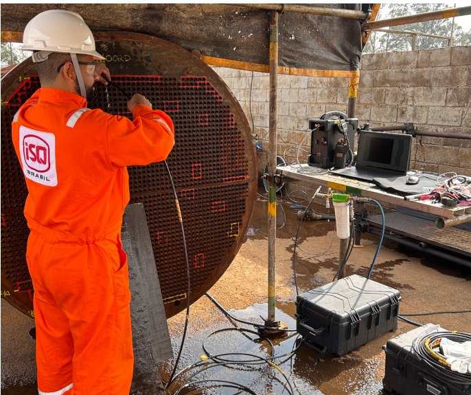
Figure 4: Heat exchanger inspection using the internal rotary inspection system (IRIS) with Ectane 3.
