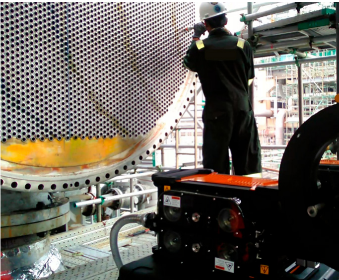
Figure 3: Heat exchanger inspection using the Probot.
