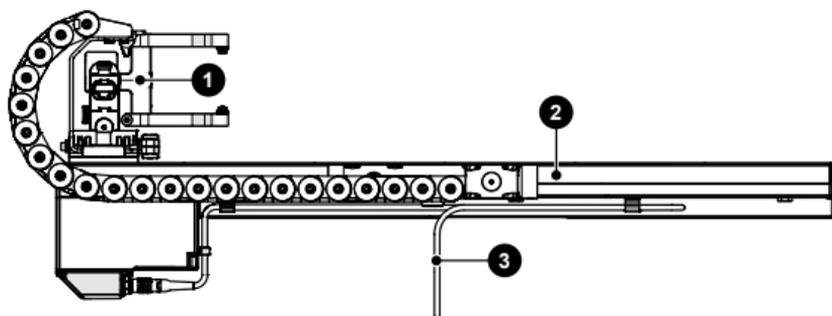
Fig. 55 - Standard Motorized Raster Arm configuration with heavy duty vertical probe holder
