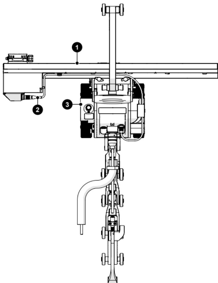
Fig. 46 - Standard MOTIX Motorized Raster Arm configuration
