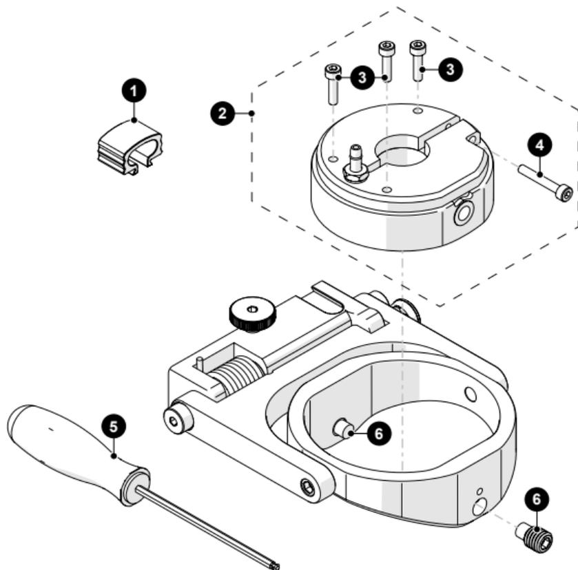
Fig. 166 - Corrosion thickness probe holder parts
