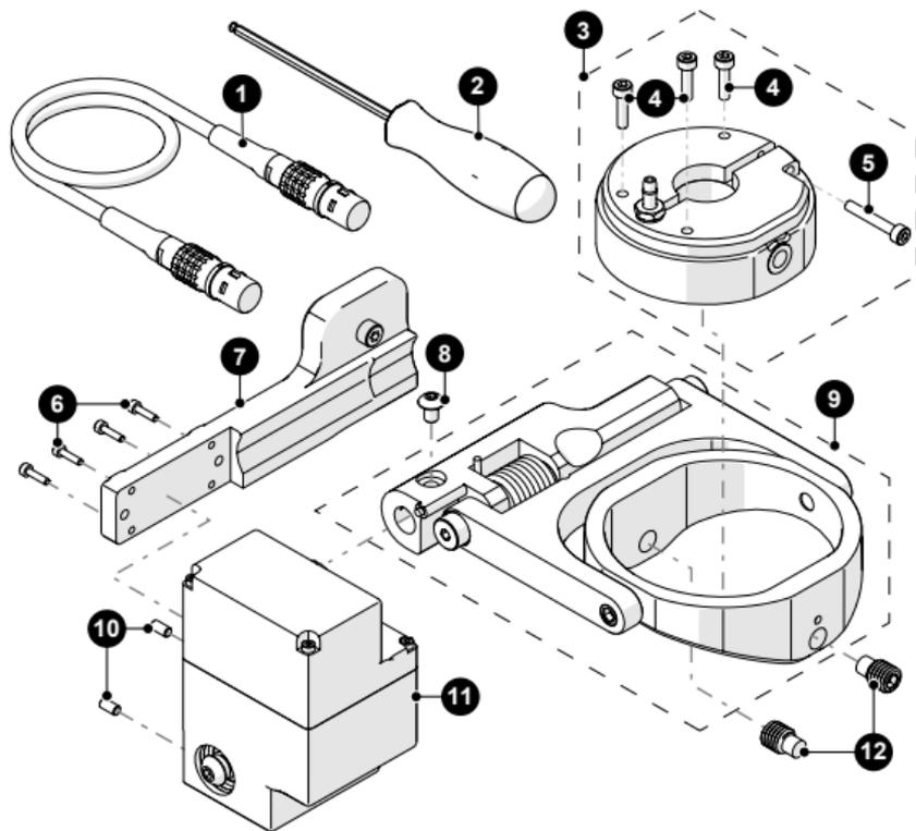
Fig. 167 - Raster arm actuated probe lift
