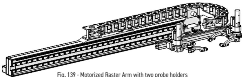
Fig. 139 - Motorized Raster Arm with two probe holders
