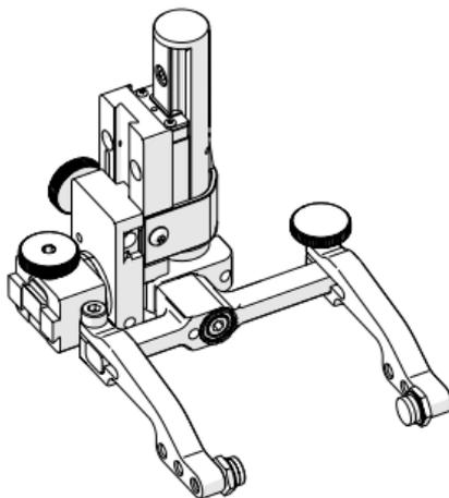
Fig. 87 - Reversed probe holder
