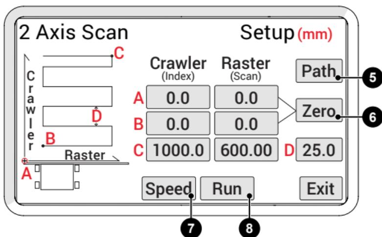
Fig. 148 - 2 axis scan setup
