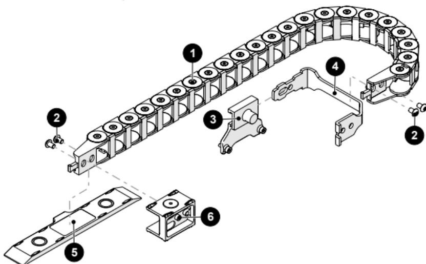
Fig. 160 - Cable tray parts
