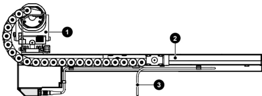
Fig. 54 - Standard Motorized Raster Arm configuration with corrosion thickness probe holder
