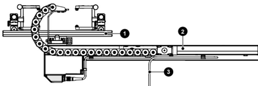
Fig. 57 - Standard Motorized Raster Arm configuration with dual probe holder
