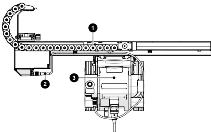
Fig. 38 - Standard SKOOT Motorized Raster Arm configuration
