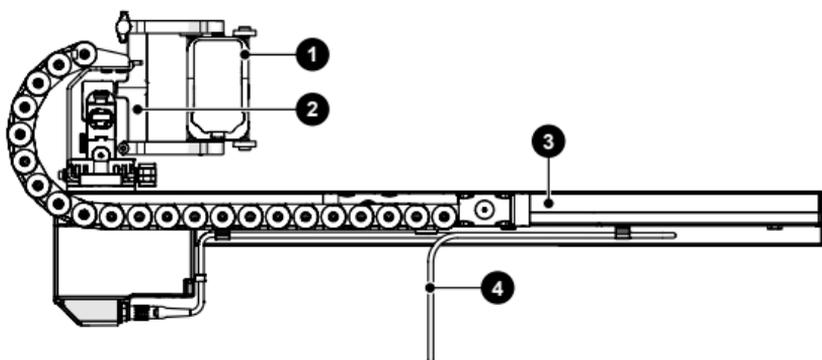
Fig. 56 - Standard Motorized Raster Arm with heavy duty vertical probe holder & HydroFORM cart
