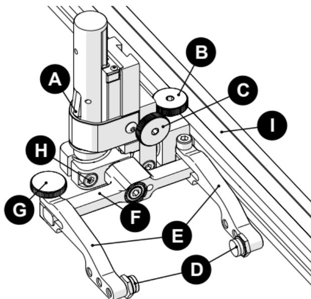
Fig. 63 - Vertical probe holder
