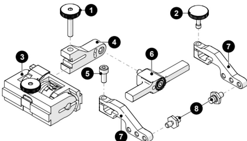
Fig. 164 - Slip joint probe holder parts
