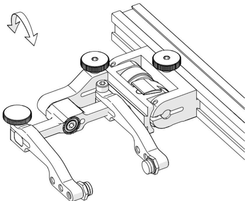
Fig. 111 - Reversed probe holder
