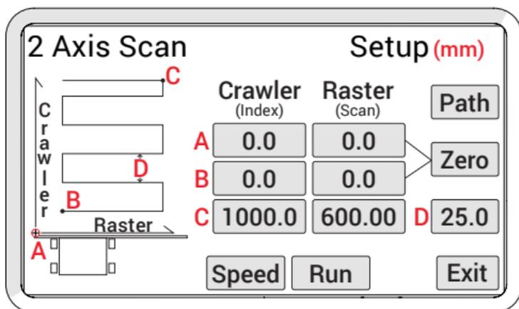
Fig. 147 - 2 axis scan setup
