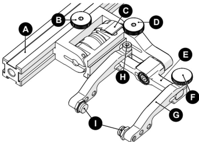
Fig. 88 - Slip Joint Probe Holder
