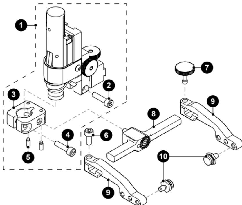
Fig. 163 - Vertical probe holder parts
