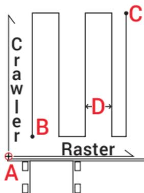
Fig. 150 - Crawler scan direction
