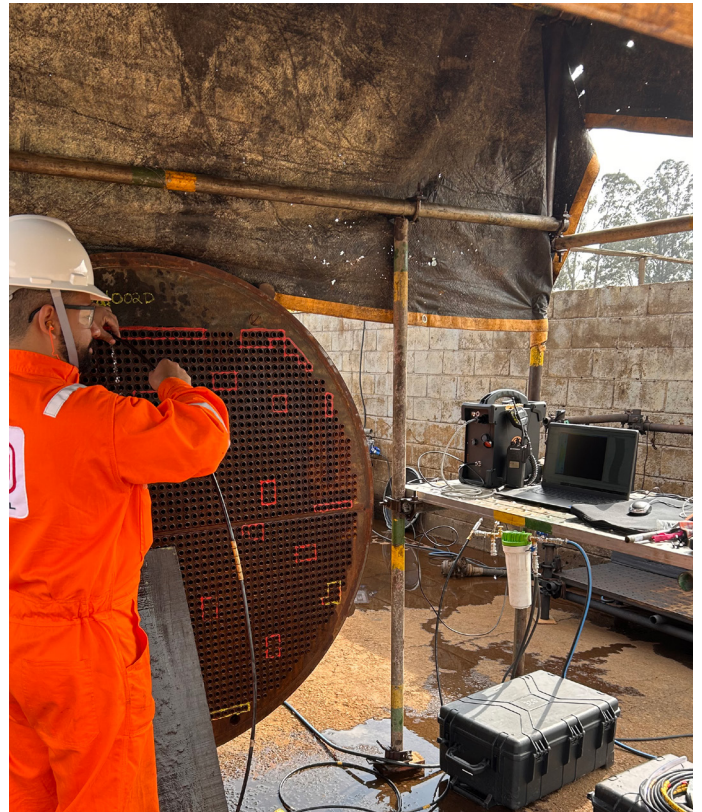
Figure 3: Heat exchanger inspection using a DefHi ECA probe paired with the Ectane.
