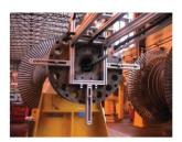
can be difficult and timeconsuming because of the length and diameter of the rotors. Eddyfi Technologies developed a system used by many in the industry to inspect bores with a combination of ECA and UT.
