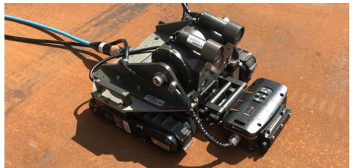
Figure 4: NDT series based on magnetic platform featuring an eddy current array probe.
