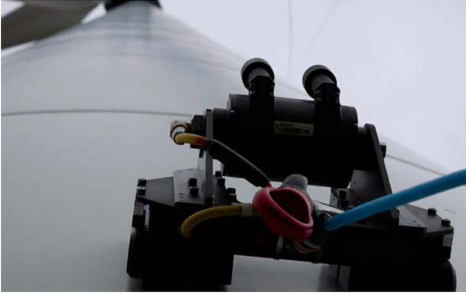
Figure 1: VT-M310, medium class crawler, designed for tank inspections, vessel inspections, wind tower inspections, and weld inspections.
