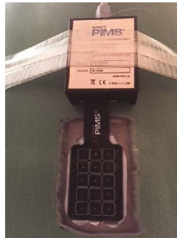
Figure 3: matPIMS™ 3x5 matrix permanently installed with RS-485 cable back to surface for data collection, pre-overwrap.
