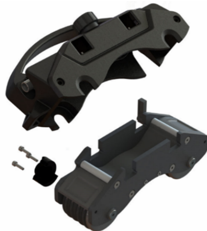
Figure 38: Encoder replacement step 3
