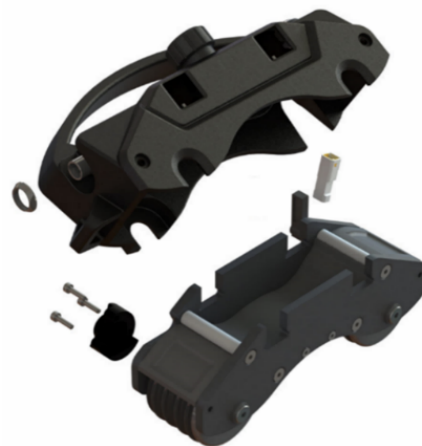
Figure 39: Encoder replacement step 4
