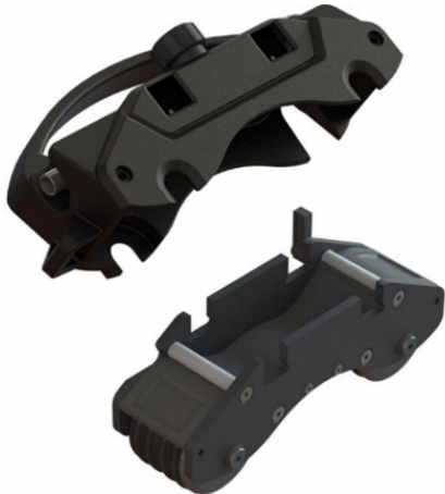
Figure 37: Encoder replacement step 2
