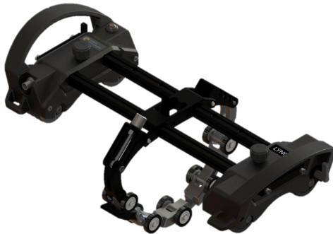
Figure 29: LYNCS CHAIN and scanner configuration with two tractors
